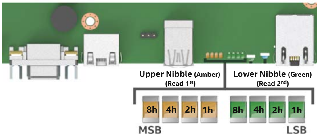
Figure 95. Onboard POST diagnostic LEDs
