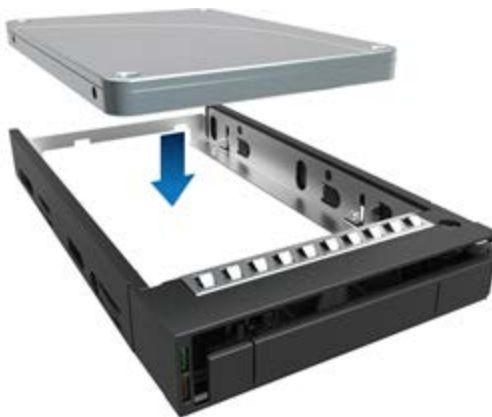
Figure 44. Hot swap drive carrier
