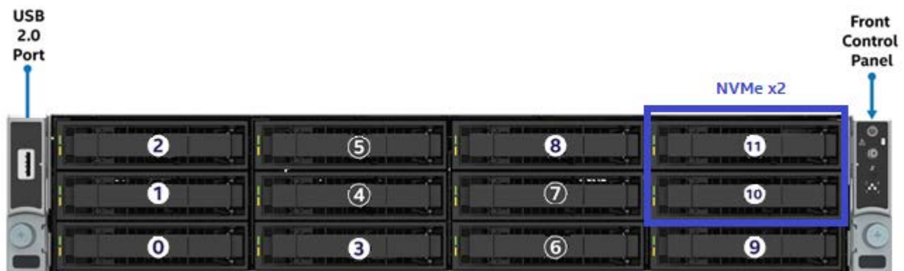
Figure 43. 3.5" drive bay, 12-drive configuration
